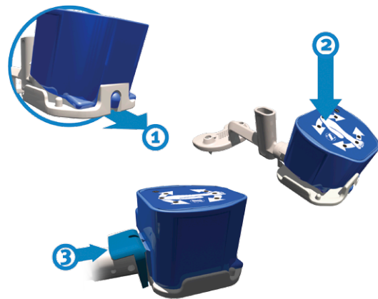
Figure 3.2 – Assembling a Pod to an Instrument
