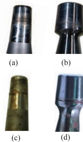
Figure 5 — Laboratory taper observations (a,b) representing accelerated corrosion fatigue test that most closely replicated the upper bound of clinical observations (c,d) of the Ti-6Al-4V 6 degree and 12/14 head/stem tapers.
