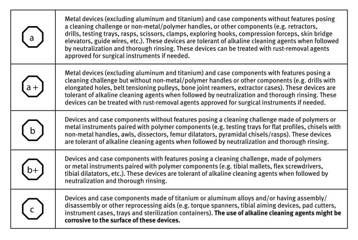
Note: Features posing a cleaning challenge include: lumens/cannulated bores, tightly mated surfaces, rough surfaces, ball detents, springs, and multiple component designs.
