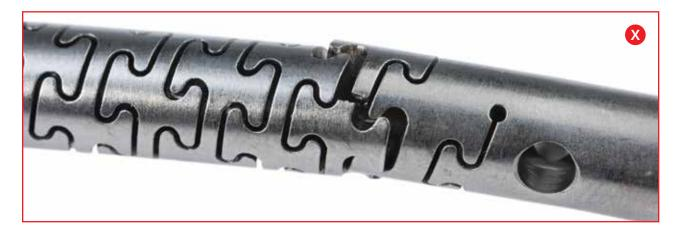
• Cracked/Fractured in flexible shaft body
