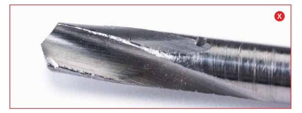
• Damaged cutting edges
