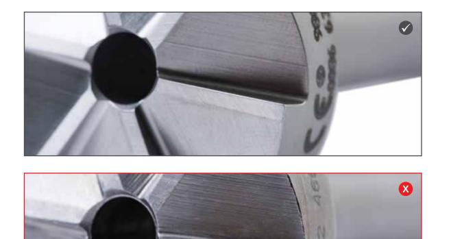
• Damaged cutting edges
