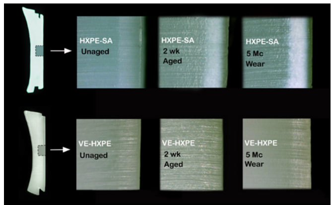
Figure 27. Cross section films of HXPE-SA and VE-HXPE unaged, accelerated aged and 5.0 Mc of wear testing. 65
