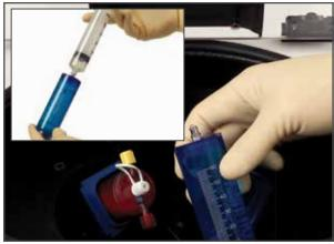
Fill GPS® III counterbalance (800-0508) with 60 ml of sterile saline and place into opposite side of centrifuge.
