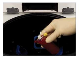
Push Open/Stop button on control panel. The "unlocked" indicator will illuminate. Turn latch counterclockwise to open lid. Place tube into centrifuge.
