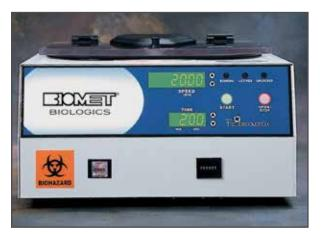
Plasmax® Plus: Place concentrator into centrifuge with the empty Plasmax® Plus counterbalance (800–0512). They should be placed on opposite sides in the centrifuge. Spin for 2 minutes at 2000 RPM.
