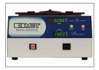
Close the lid by rotating the lid latch clockwise. "Latched" indicator will illuminate. Set speed to 3200 RPM and time to 15 minutes. Press green button to start spin. Once spin is complete, press red button to illuminate the "Unlocked" indicator. Twist latch counterclockwise to open lid.
