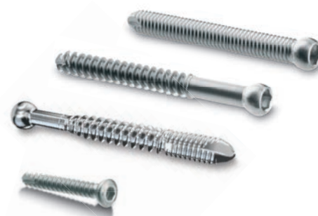
Self-tapping screws: Double lead thread for fast screw insertion in cortical bone. Ø 5.0 mm NCB cortical screws L= 14–100 mm Ø 5.0 mm NCB cancellous screws L= 50–100 mm Ø 5.0 mm NCB MotionLoc® screws L= 30–60 mm Ø 3.5 mm cortical screw L= 50–85 mm
